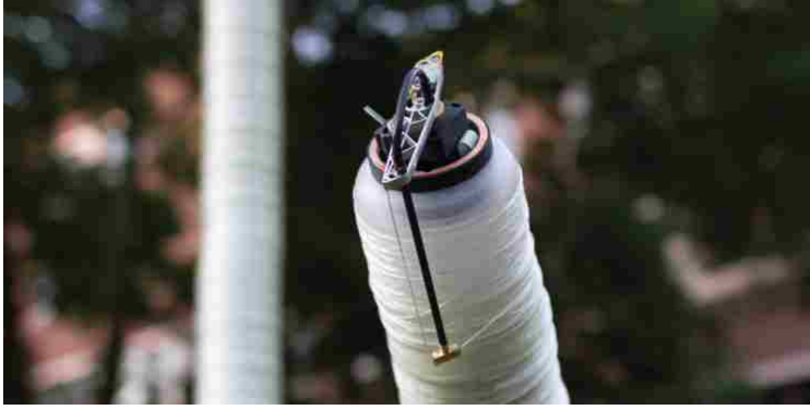
Figure 9 Fiberbot fabricating the tube – Source: The Mediated Matter Group
