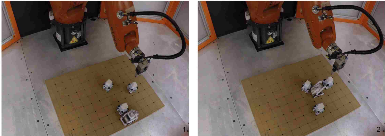
Figure 30 Obstacle avoidance of recognized objects
